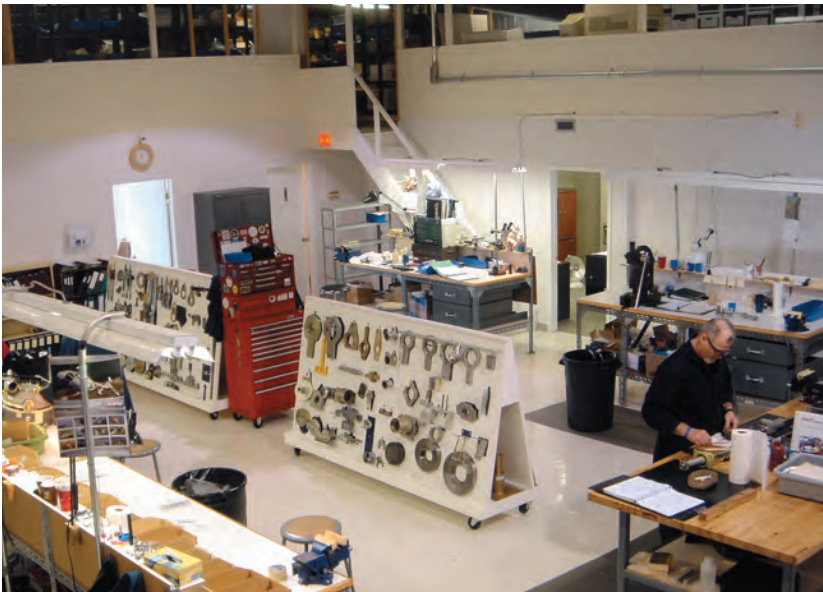
Tool array for the Bell Helicopter series of Dynamic Components in the Helitrades component assembly room. Photo courtesy of Helitrades Inc., Vankleek Hill, ON.
